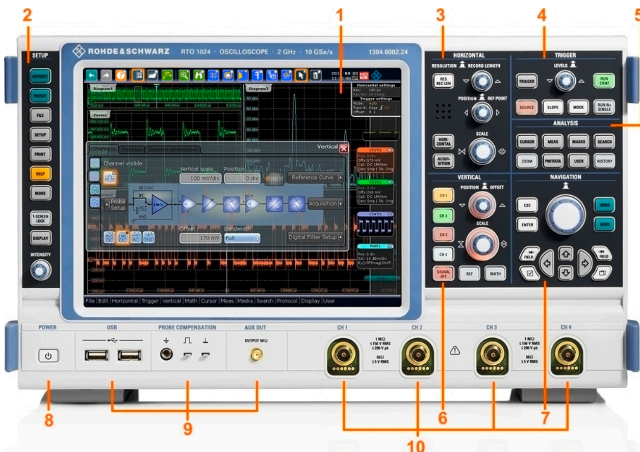
Fig. 3-1: Front panel of R&S RTO1024 with 4 input channels
